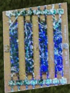
SAW Biosensor for Optikus™ pathogen detection
