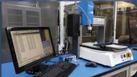
Robotic assembly workstation for fabrication of microfluidic components
