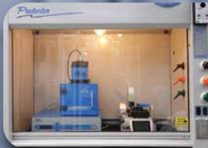
UV Oven used to cure microfluidic components to prevent contamination
