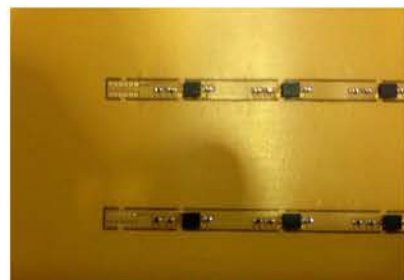
MOSFET Sensor Module dimensions: 1x1.2x0.3mm
