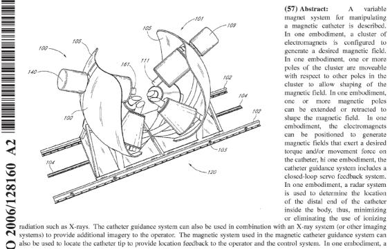
(57) Abstract: Α variable magnet system for manipulating a magnetic catheter is described. In one embodiment, a cluster of electromagnets is configured to generate a desired magnetic field. In one embodiment, one or more poles of the cluster are moveable with respect to other poles in the cluster to allow shaping of the magnetic field. In one embodiment, one or more magnetic poles can be extended or retracted to
